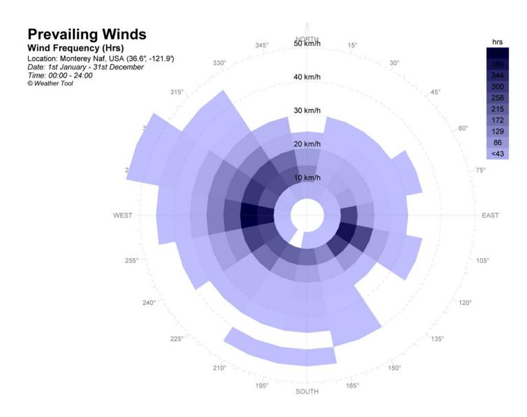
**Wind Analysis**: The graphs above were calculated with the climate analysis software Ecotect and represent the average yearly wind speeds and directions for the Winter, Summer, Spring, and Fall in Monterey California. Generally, a cool prevailing wind is present from the North / North West direction with a speed of 10 to 30 km/hr. or 6 to 18 mph.
