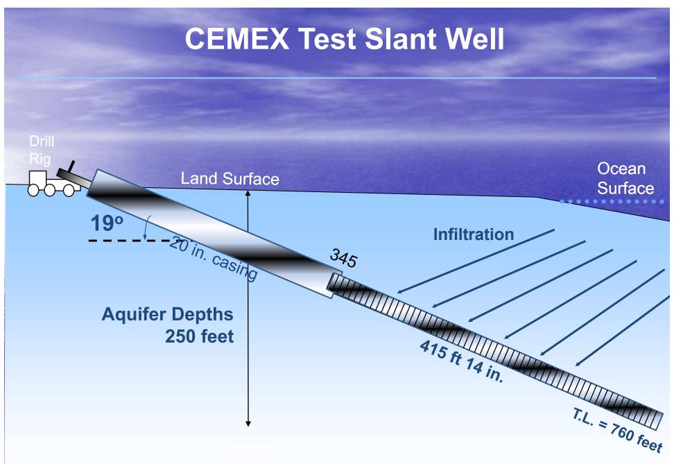
\* Larger test well casing allows full development of the well (1.5 x the design capacity) unlike Dana Point well
