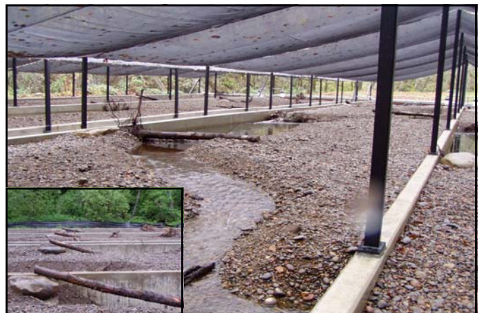
Shade cloth suspended above the artificial streams to replicate shade.
