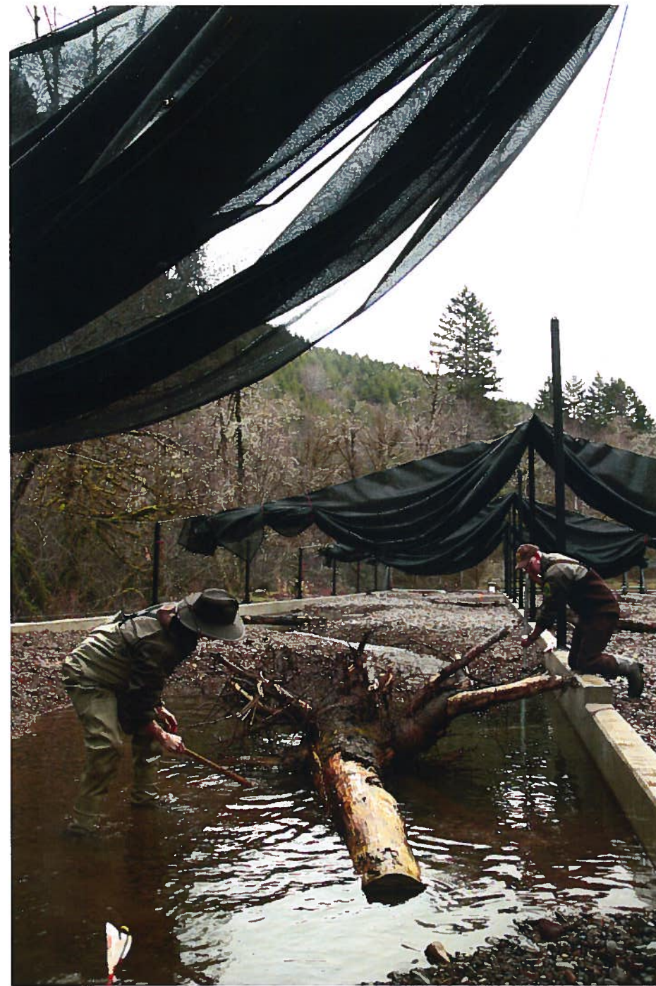
Experimental streams mimic natural features with gravel bars, woody debris, and natural meanders and pools.
