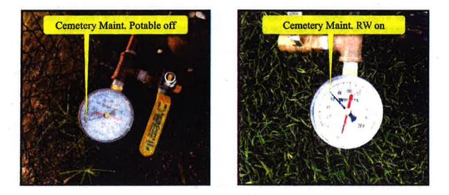
Following confirmation that shutting down the potable service did not impact any RW outlets the potable service was restored at the potable RP and the RW system in this area was shut down at 1635. It was then confirmed that only the RW outlets were off and the potable system remained pressurized at this part of the test. This took place at 1650. See pressure gauge images on next page. No cross connections were discovered in this area.
