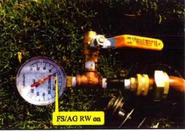
Following confirmation that all outlets on both systems were confirmed to be on, the potable systems were shutdown at the potable RP services to Crespi and the FS/AG at 1012.
