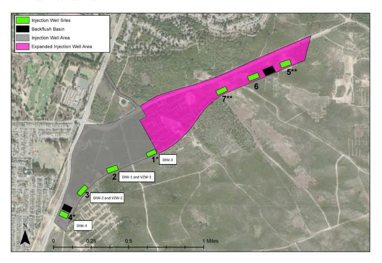
Well sites 1-4 have been approved and constructed. Well site 6 is the primary site for expansion, but sites 5 and 7 may be made available for redundancy or future replacement.
