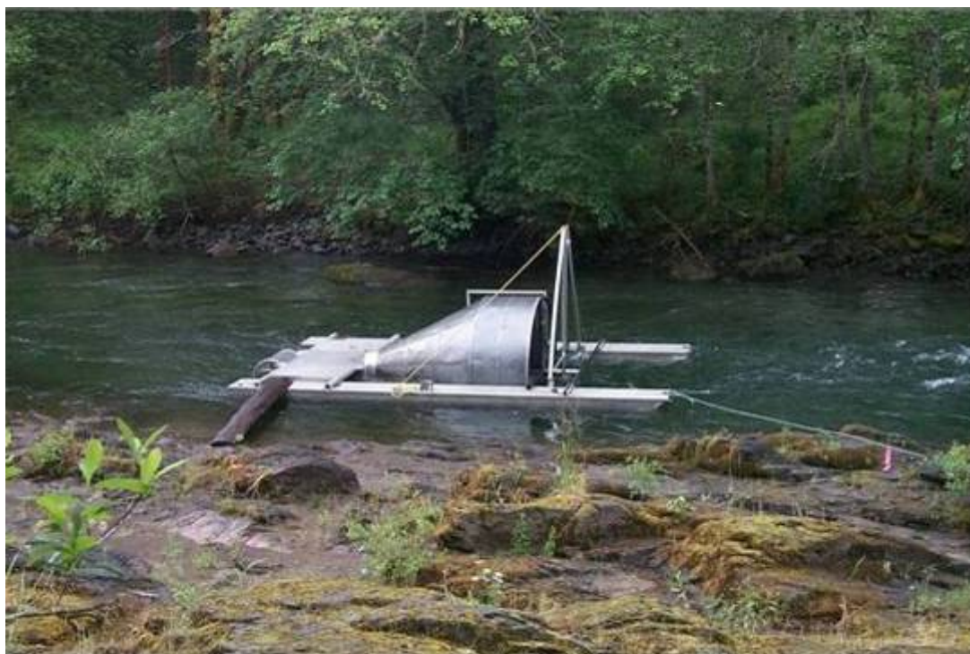
Figure 13. Photograph of typical screw trap that may be used at the reservoir inlet.
