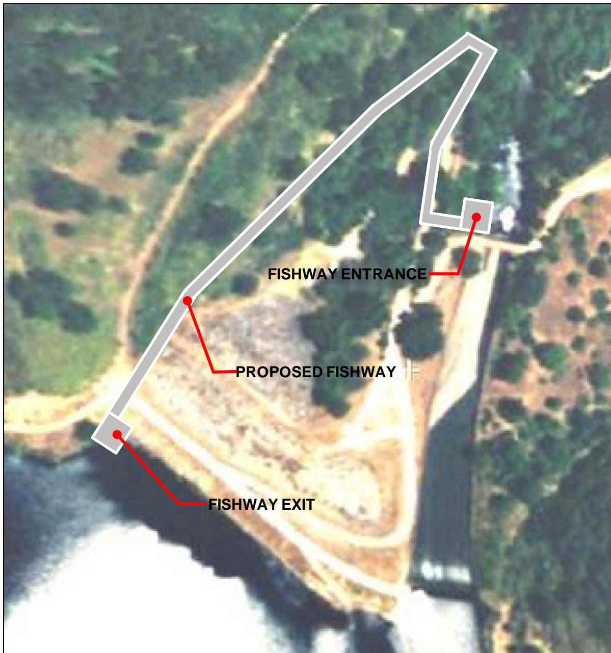
Figure 9. Schematic of hybrid vertical slot fishway extending from tailrace to reservoir forebay.
