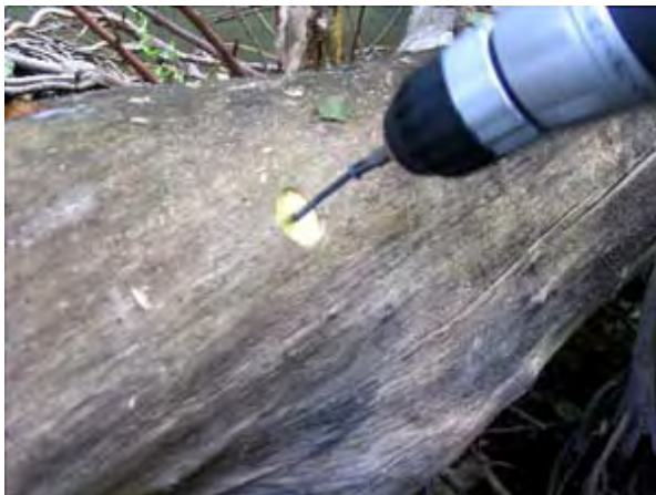
Figure 2: Attaching an identifying tag to a piece of LWD
